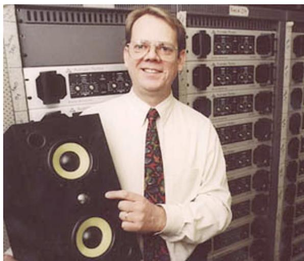
A new Australian Monitor amplifier was developed based on the well-known AM1200 workhorse with an on-board microprocessor and in-built Cresnet computer network interface for control and monitoring. The 51 amplifiers are conservatively rated at 4 x 200W each for a total system power of more than 40,000W.
