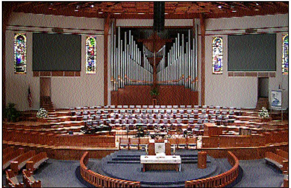
***The choir loft canopy produces reflections that are almost at echo threshold. Enhancement created a “virtual canopy” for the choir.***
